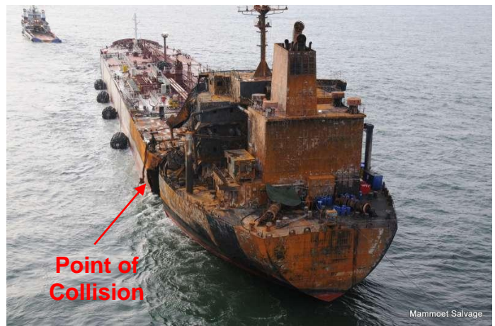
Formosaproduct Brick Fire and Structural Damage
