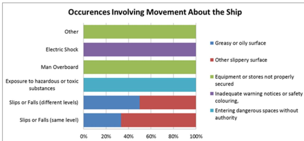
The chart above shows that the predominant "movement about the ship" cause has been attributed to 'other' slippery surfaces and "equipment or stores not properly secured". Where appropriate masters should ensure that deck working areas have non-slip surfaces. This can be achieved by either clearing/cleaning the deck, placing non-slip mats or use of non-slip paint mixes. Crew members should also be aware of any associated risks of slipping when moving about the ship under various conditions.
