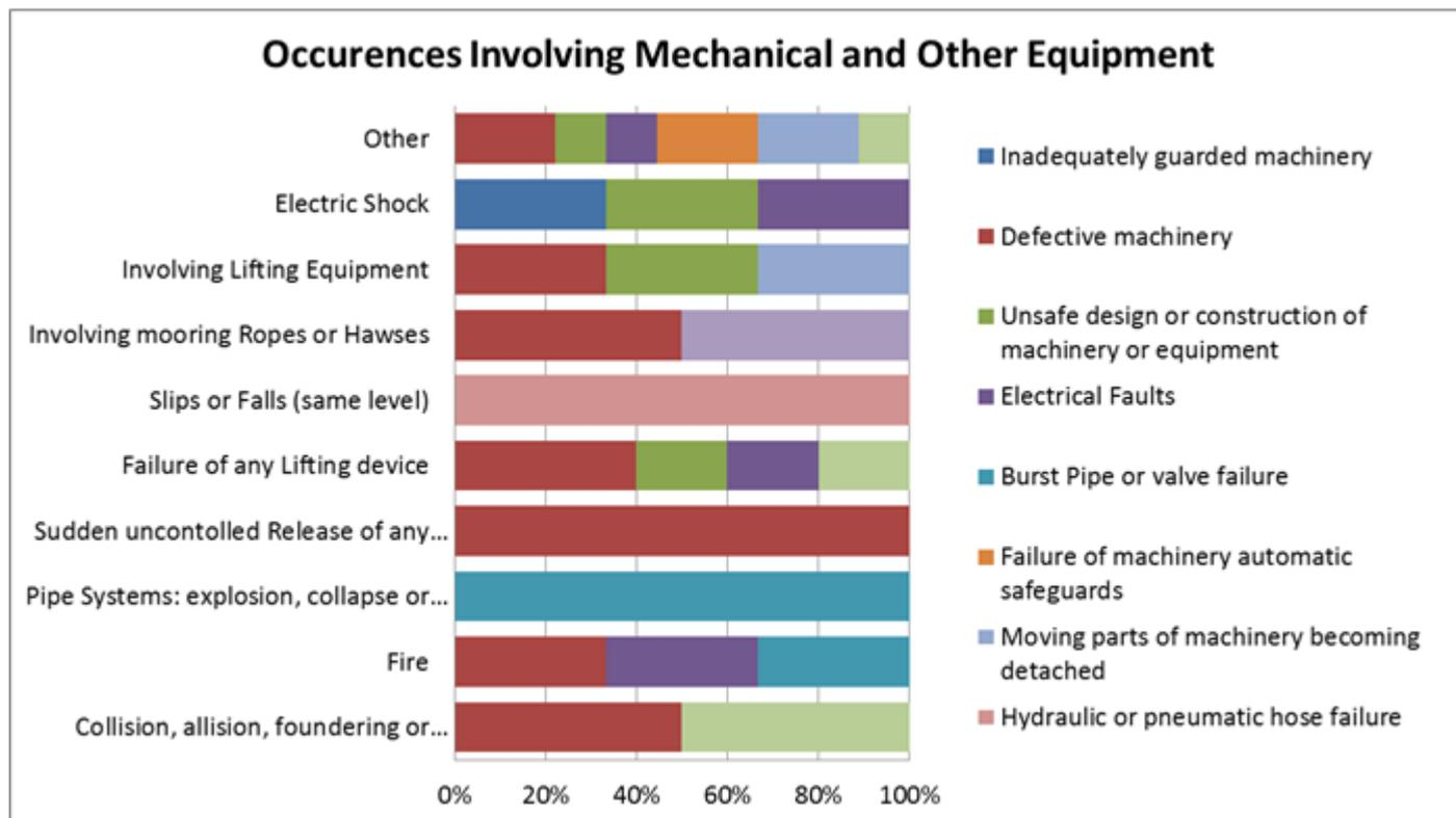
The chart above shows an approximately even spread with various mechanical, electrical, ropes and associated equipment malfunctioning. This stresses the need for effective inspection and maintenance to ensure they are in good condition and fit for purpose.
