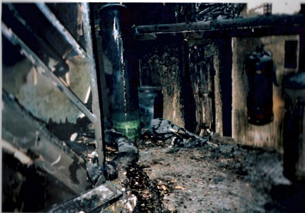
Fire damage at stairwell access from engine room to deck
