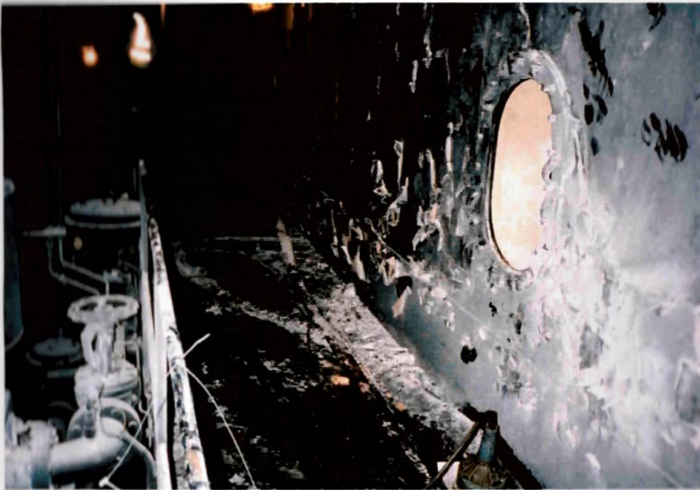
Fire damage at walkway by base oil tank manhole at outer starboard side of starboard main engine
