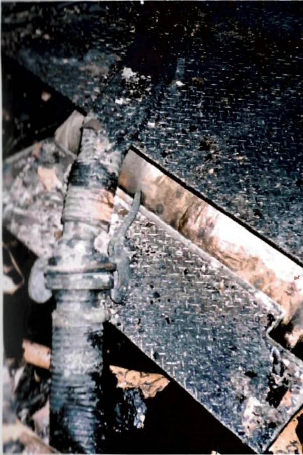
Base oil hose remains with connections at bottom of deck stairwell
