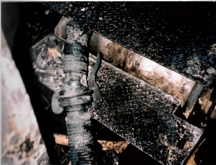
Base oil hose remains with connections at bottom of deck stairwell
