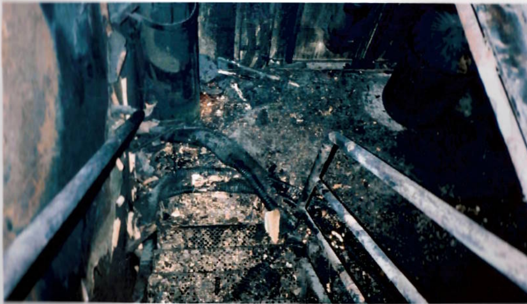
Fire damage at stairwell access from engine room to deck
