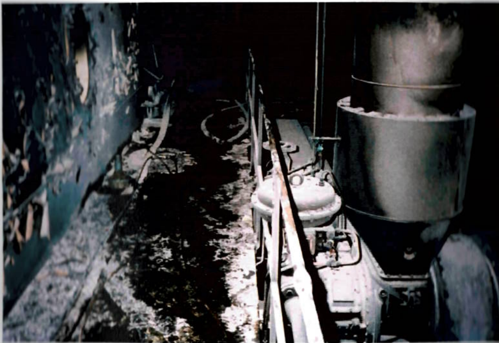
Fire damage at walkway by base oil tank manhole at outer starboard side of starboard main engine
